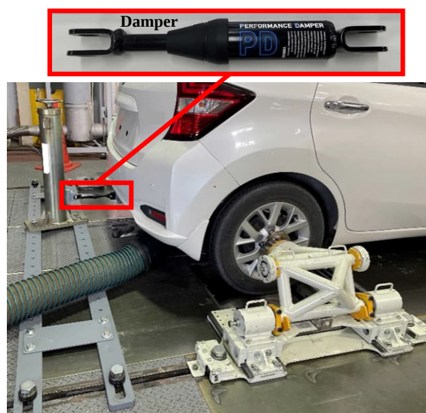
Fig.2 The Damper Implementation
