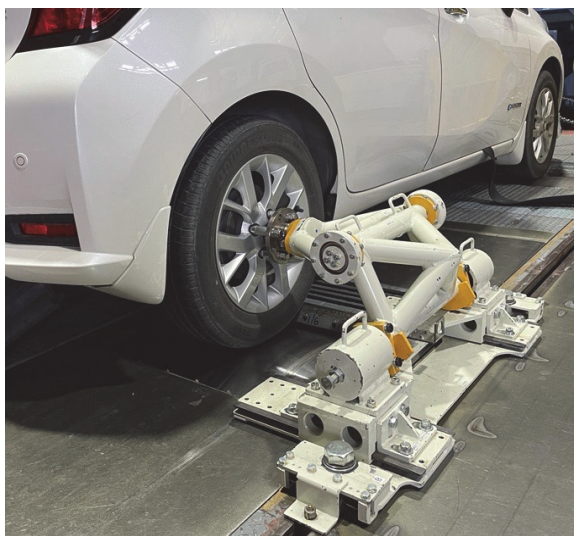
Fig.1 Hub Nut Clamp Type Vehicle Restraint Device
